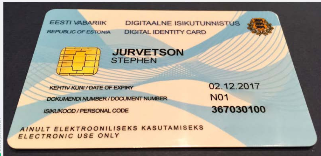
Enlarge / 750,000 Estonian cards that look like this use a 2048-bit RSA key that can be factored in a matter of days.
